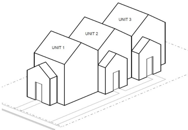
Figure 22.285-3. Duplex Attached by Breezeway
