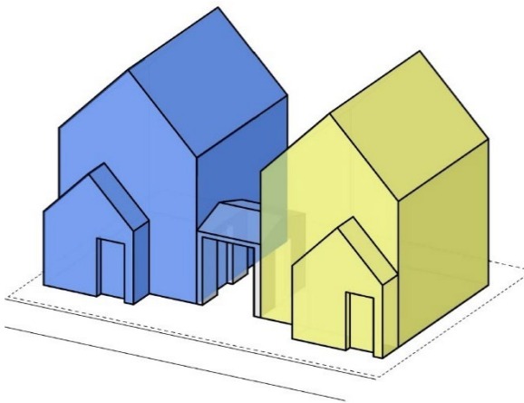
Figure 22.285-3. Duplex Attached by Breezeway
